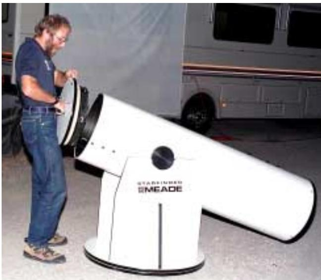
*Weber State University astronomer John Sohl removes the primary mirror from a Meade 16" reflector. Note the simple-but-strong "Dobsonian" *alta-azimuth* mount. Six or eight-inch reflecting telescopes on Dobsonian mounts make excellent first telescopes.*
