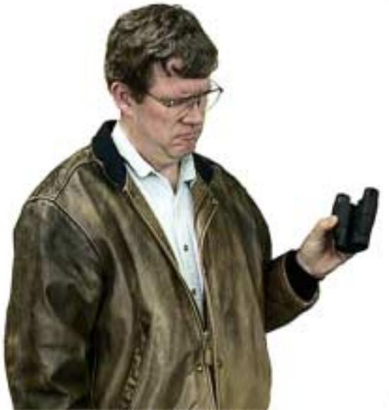
*Small binoculars such as this set of 8x25's (8 power magnification, 25 mm apertures) may work well in daylight but don't gather enough light for use at night.*
