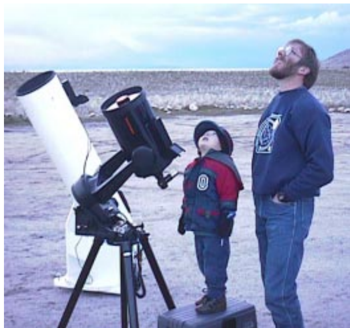
Schmidt-Cassegrain telescopes (foreground) are compact reflector telescopes, that use its secondary mirror to reflect light to the rear of the telescope.
