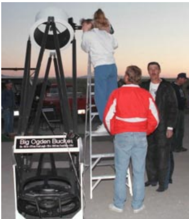
Meet BOB: The "Big Ogden Bucket" 18-inch reflector owned by the Ogden Astronomical Society. Note that this telescope uses removable braces, instead of a solid tube, to hold the secondary mirror and eyepiece.
