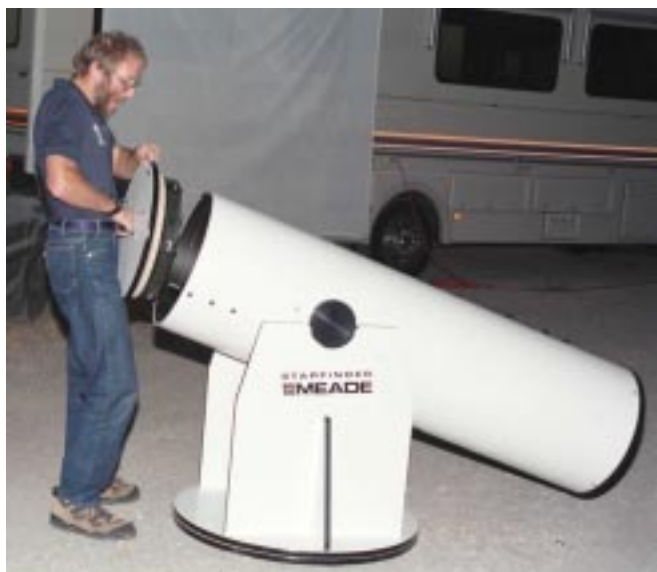
Weber State University astronomer John Sohl removes the primary mirror from a Meade 16" reflector. Note the simple-but-strong "Dobsonian" alt-azimuth mount. Six or eight-inch reflecting telescopes on Dobsonian mounts make excellent first telescopes.
