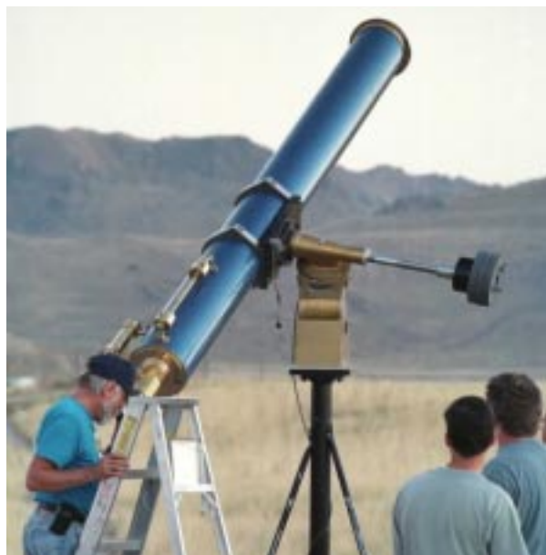
Refractors are capable of producing sharper images than reflecting telescopes of the same aperture, but are big, heavy and expensive. Siegfried Jachmann's nine-inch Clark Refractor offers eye-popping views of the planets, but taking it to a Star Party is not a simple task.
